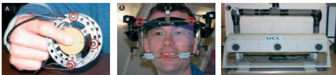
Fig. 5. The experimental platform includes (A) two force-torque transducers measuring the full six components of force and torque ( F_x, F_y, F_z, T_x, T_y, T_z ), (B) a Chronos video-based 3-D binocular eye movement recording system, (C) a 3-D movement tracking system measuring the kinematics of the instrumented object grasped between the fingers and the Chronos helmet (note the LEDs inside the red circles).
