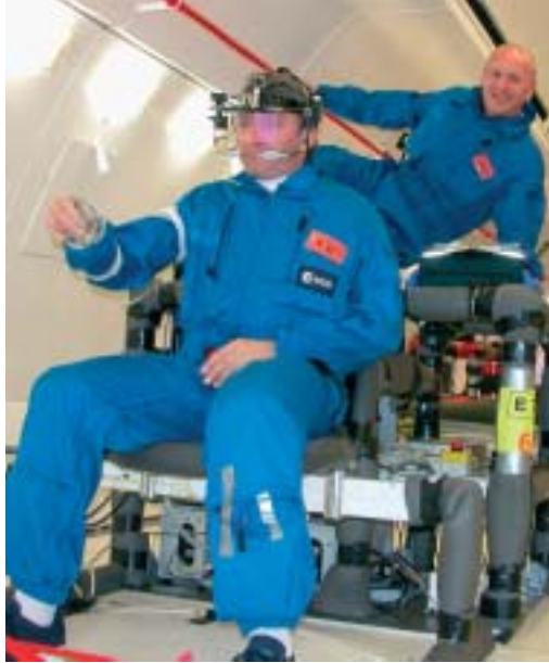
Fig. 6. Frontal view of the experimental set-up. The subject is secured by a seat belt on a chair, with the instrumented object grasped, in the frontal plane, between the thumb and the index finger of the right hand. On a signal 20 s before the 1.8 g pull-up phase, the subject is requested to move the object continuously in a figure of '∞'.
